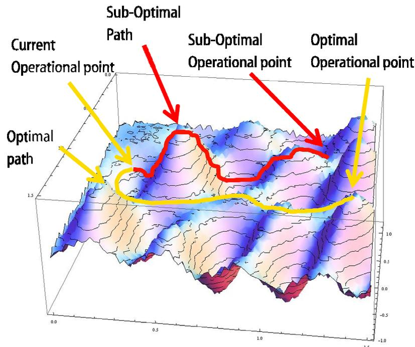
**Figure 3.:** The dependency of the goal on two controllable variables. The upper path displays the reaction of a human operator and the lower path displays the reaction of the optimization system. The paths are different and arrive at a different destination. The optimized path is better than the human determined path by approximately 5% as measured by the goal function.
