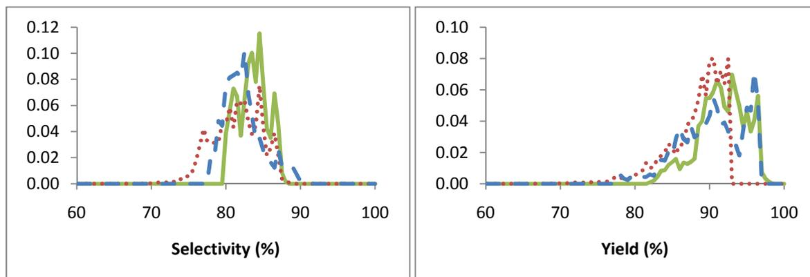
**Figure 4.:** The probability distribution functions for selectivity and yield of  $D_i$  for periods in which the optimization was not used (dotted), used for controllable variables without the catalyst (dashed) and used fully without restrictions (solid).
