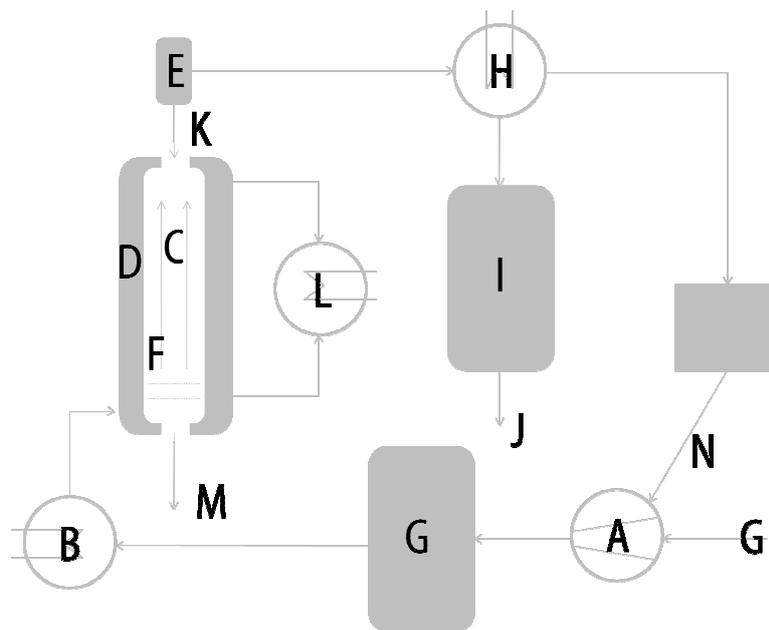
**Figure 1.:** Sketch for the Müller-Rochow-Synthesis plant including: (A) Compressor, (B) Vaporizer, (C) Fluidized bed reactor, (D) Cooling jacket, (E) Cyclone, (F) Silicon / Copper (catalyst), (G) Methyl chloride, (H) Condenser, (I) Raw Silane, (J) To the distillation, (K) Silicon / Copper dust, (L) Heat exchanger, (M) Remainder, and (N) Backflow methyl chloride.
